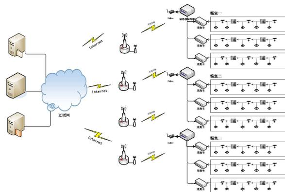
Fig. 1. Greenhouse film monitoring network scheme
